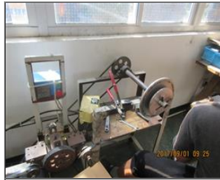
Photo of non-conformity No safeguarded 1.JPG
