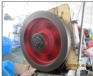
Photo of non-conformity No safeguarded 2.JPG
